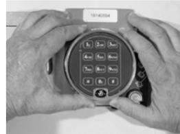
12. Place the keypad over the base. Make sure the keypad cable is clear of the pad's two spring clips as you push the keypad firmly onto the base. It should snap into place. If you need to remove the keypad, pull the bottom (area nearest the S&G logo) away from the mounting base first. Never allow the keypad to hang by the attached cable. The installation is complete, but do not close the safe door until successfully completing the following lock test.
