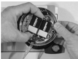
10. At the front of the safe, install a new 9-volt battery in each of the keypad's two battery holders. Duracell® brand batteries are recommended. **Support the top of each holder with a thumb or finger as each battery is inserted. This will help prevent bending or breaking the holder posts.**
